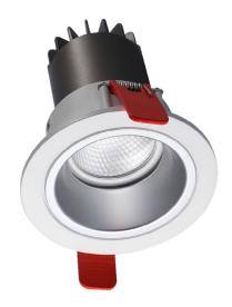
The Maia LED is a 130mm diameter downlight which uses a CREE LED engine. The heatsink is constructed from die-cast aluminium complete with aluminium bezel and reflector. The bezel features a 40mm recess detail which can be finished in gold, silver or chrome effect.
