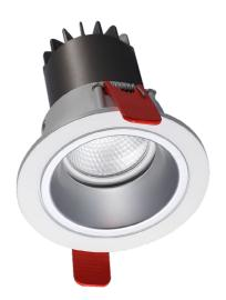
The Maia High Output LED is a 130mm diameter downlight which uses a Citizen COB LED engine. The heatsink is constructed from die-cast aluminium complete with aluminium bezel and reflector. The bezel features a 40mm recess detail which can be finished in gold, silver or chrome effect.
