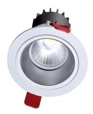
The Maia Mini LED is a 90mm diameter downlight which uses a CREE LED engine. The heatsink is constructed from die-cast aluminium complete with aluminium bezel and reflector. The bezel features a 40mm recess detail which can be finished in gold, silver or chrome effect.
